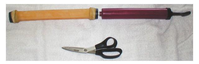
To try to stretch the center portion of a section of liner material by inflation, you need to first seal the cut length up on both ends. One thing that works well for this is a pair of rubber stoppers, one solid and one with a single hole in it. Note they are installed backwards, fat end first, for a better grip, and held firmly with rubber bands.
