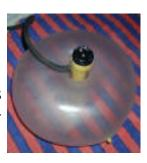
Inflating a Geo around a receiver is one case in which you may want to make up the receiver with the hose tubulation at the back or cap end of the housing. This allows the front to be free of the hose for a better fit on that side. Putting the hose on the rear of the housing does give the hose a greater opportunity to pull sideways on the receiver, so it is a tradeoff.
