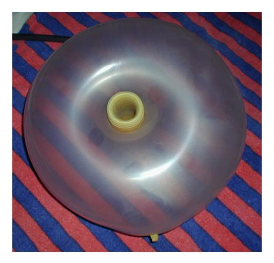
This is one case where mounting the hose tubulation at the rear of the housing could be an advantage. But the Geo balloon support works either way. This is not really a practical solution to the face down receiver problem. The hard receiver is still a major factor in any attempt to use the receiver face down without lots of padding underneath it and there is danger the balloon might burst, so face down use cannot be recommended.
