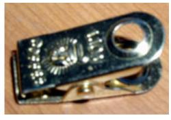
I had also drilled a hole in the new combined base in a convenient place so I could mount the clip near the center of balance. I have found these clips in several places. Sometimes used to reseal bags of fancy coffee or tea. Often the perfect clips are found on nametags. They have "buck teeth", that is one jaw overlaps the other as they close, which makes them particularly effective in grabbing clothing or sheets. The ones from nametags often have nice
